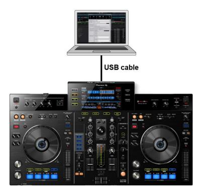
Connect your PC/Mac and an all-in-one DJ system using a USB cable.
