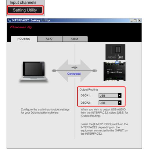
10 Check the settings in [Output channels]. Play a track on a deck on rekordbox, monitor the sound from the DJM. If the setting is not the one you wish, change it.
