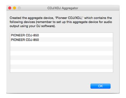
Depending on USB connection status, the aggregate device may not be created correctly or tracks may not be played properly from the created aggregate device. This might be due to band width of a USB bus or USB hub on the Mac connected to CDJ/XDJ. The same thing may happen even if you do not use the CDJ/XDJ Aggregator and create an aggregate device by Audio MIDI setting (Mac OS). Please rename the aggregator as "Pioneer CDJ/XDJ".
