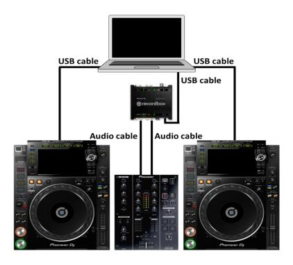
This section describes how to set up connection with a stand-alone audio interface as an audio device. Install driver software before connection as described in 1.2.2 Driver installation.
